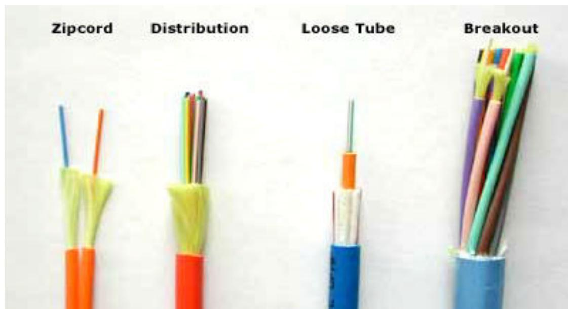
**Simplex and zip cord:** Simplex cables are one fiber, tight-buffered (coated with a 900 micron buffer over the primary buffer coating) with Kevlar (aramid fiber) strength members and jacketed for indoor use. The jacket is usually 3mm (1/8 in.) diameter. Zipcord is simply two of these joined with a thin web. It's used mostly for patch cord and backplane applications, but zipcord can also be used for desktop connections.
